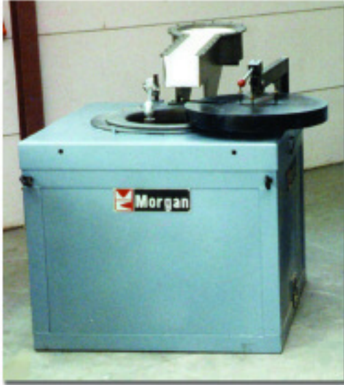
▲ Morgan's Electric Resistance Bale Out Furnace.
